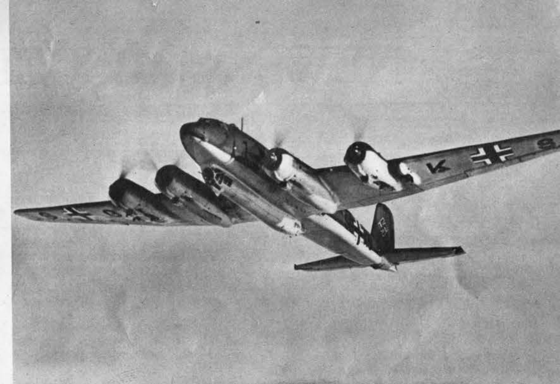
FW-200'S UNDERSIDE IS FLAT, WITH LONG OFF-CENTER BOMB BAY. TAILPLANE IS SQUARED OFF
